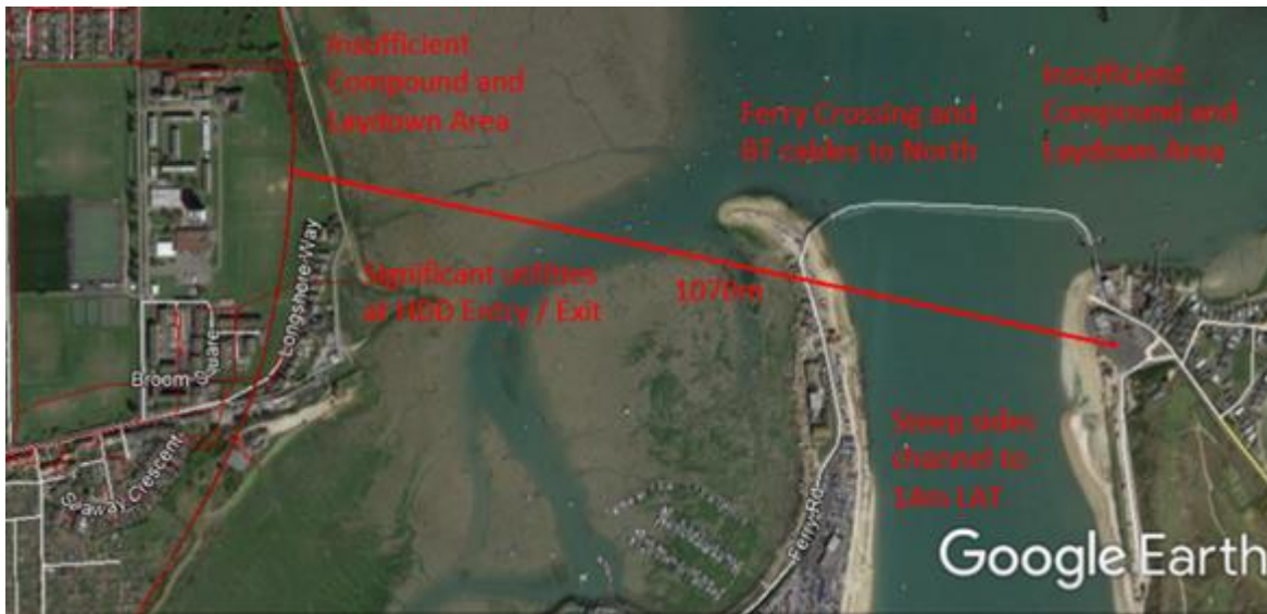
Plate 10 - Indicative HDD crossing across the Langstone Harbour entrance channel to Hayling Island
